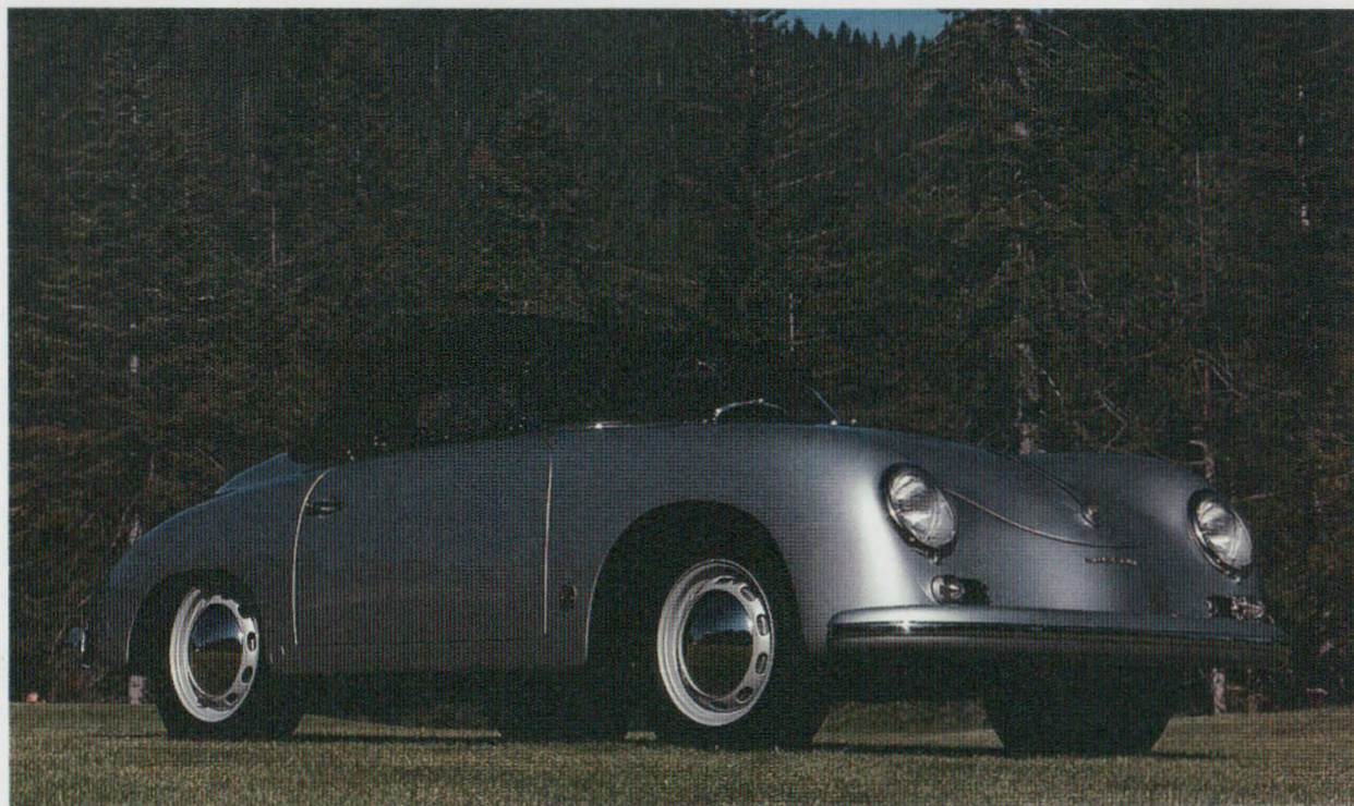
Cheryl Dunkel's 1958 Carrera GS/GT Speedster is a highly-developed version of Porsche's simple sport roadster. With a four-cam engine and many aluminum panels, it was a true dual-purpose machine for cruising and competition.
