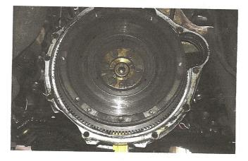
Once Nolan lowered the old four-speed down, he methodically removed all the remaining pieces attached to the rear of the engine, starting with the flywheel.
