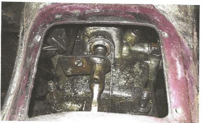
The old shifter bushings - what was left of them at all - were paper thin, which goes a long way in explaining the long and sloppy shifter throws I needed to shift from one gear to the next!
