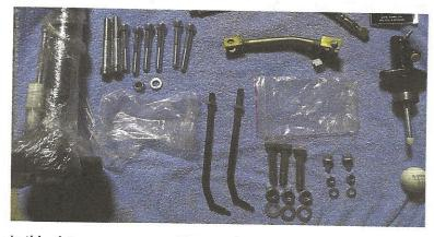
In this picture, you can see the new forward section of the driveshaft on the left, still wrapped together with the centering pin that we would be using when re-installing the flywheel, clutch plate and clutch disc.
