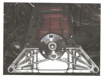
With all the parts cleaned up or replacement parts acquired, reassembly started - assembly ring adapter, flywheel, clutch disc and pressure plate were all installed. The supplied centering pin earned its keep!
