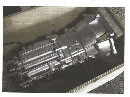
S&SG starts with a Getrag transmission and does the work of turning it into this six-speed. The workmanship and accompanying parts all had a quality feel about them. The kit included all the necessary parts to accommodate the longer length of the new transmission.
