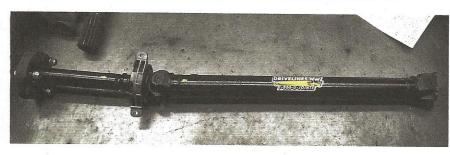
Then it was back to my mechanic to have the newly balanced combined driveshaft installed.
