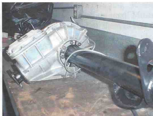
Painted and assembled 4.10 rear axle.
