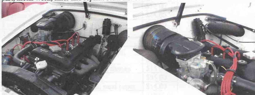
Carb and modified air filter for hood clearance.
