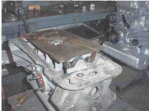
Windage tray fitted to early block
