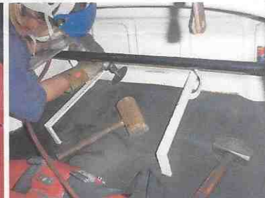
Painted weld areas. Spare tire bracket rework.
